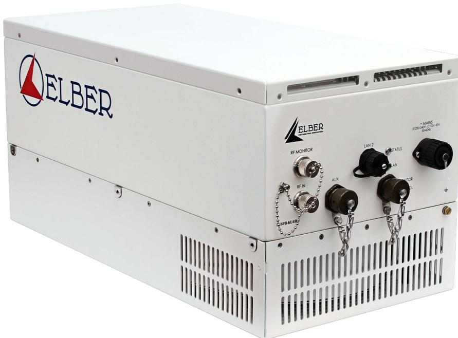
The ESSPx-Ku-2 is the outdoor solid-state power amplifiers (SSPAs) series designed and manufactured by Elber with GaN transistor technology, with output power from 100W up to 400W. Available also as SSPB, with in-house designed upconverter, the ESSPA-Ku200-2 is the 200W Ku-band version.
